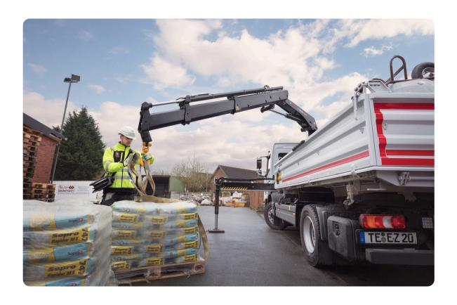
The ideal performance model within the HIAB range of loader crane products. Remote controlled loader crane. CE marked. A non CE version is also available. 11,3 Tm range capacity loader crane.
