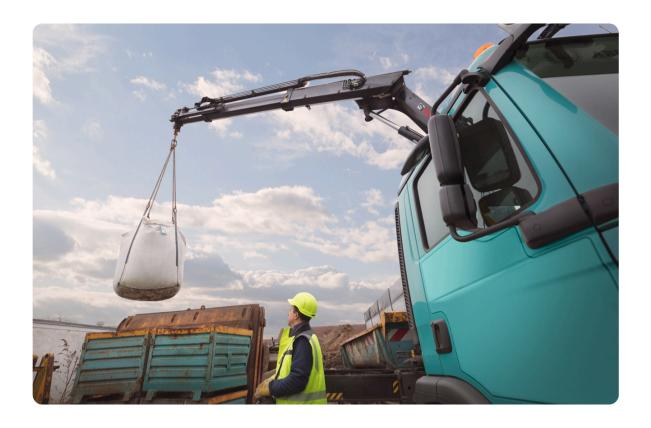
The ideal performance model within the HIAB range of loader crane products. Remote controlled loader crane. CE marked. A non CE version is also available. 10,3 Tm range capacity loader crane.
