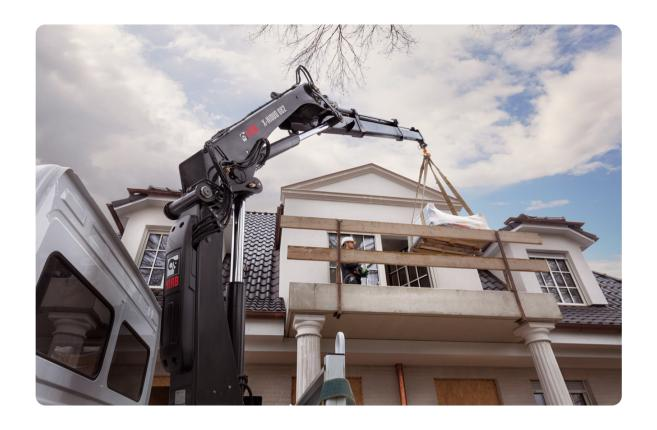
The ideal performance model within the HIAB range of loader crane products. Remote controlled loader crane. CE marked. A non CE version is also available. 8,1 Tm range capacity loader crane.
