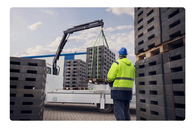
The ideal performance model within the HIAB range of loader crane products. Remote controlled loader crane. CE marked. A non CE version is also available. 6,7 Tm range capacity loader crane.
