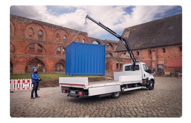
The ideal performance model within the HIAB range of loader crane products. Remote controlled loader crane. CE marked. A non CE version is also available. 4 Tm range capacity loader crane.
