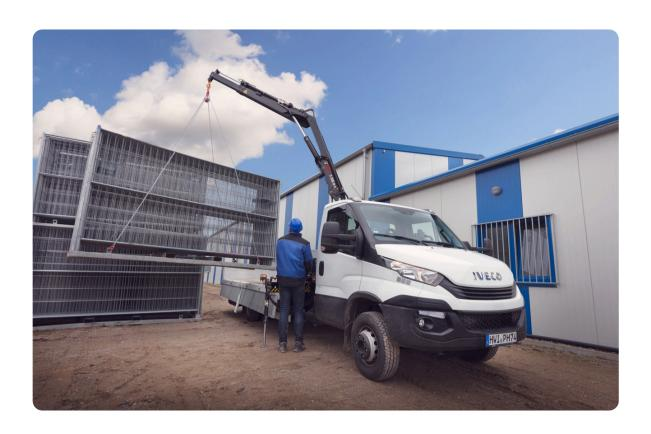
Top functions at a reasonable price point for this HIAB range of loader cranes. Manually controlled loader crane. Non CE marked. 4 Tm range capacity loader crane.
