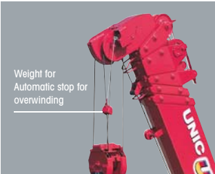
8 Automatic stop for overwinding
