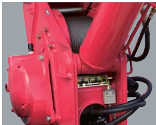
9 Automatic stop for leaving minimum wire rope
