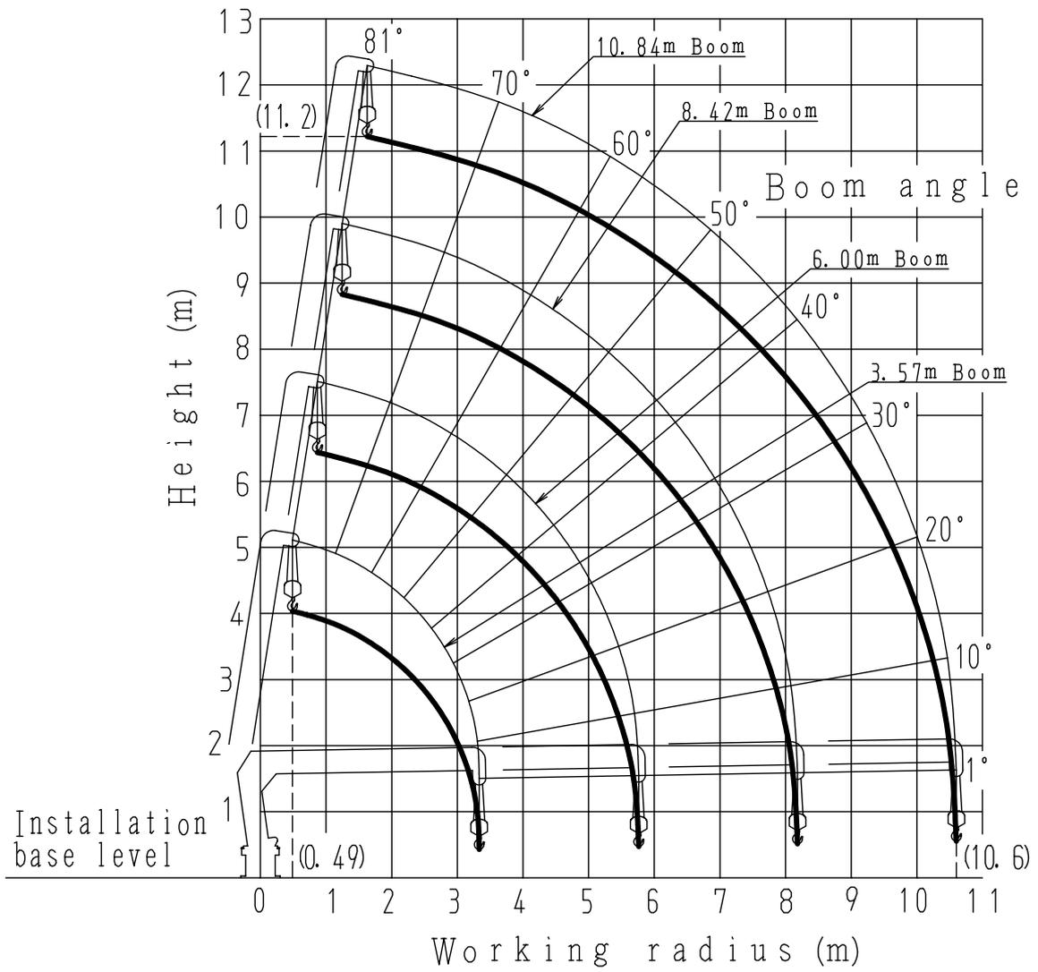
**Note:** The above figures are based on no-load condition and do not include the deflection of the boom.
