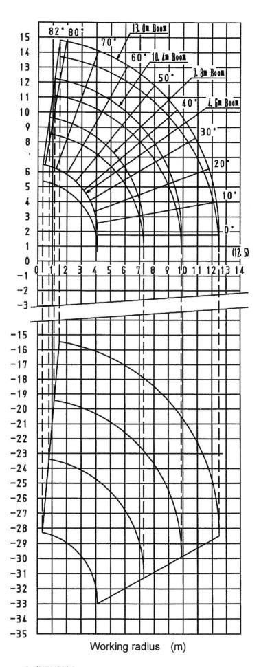
Note: The above figures are based on no-load condition and do not include the deflection of the boom
