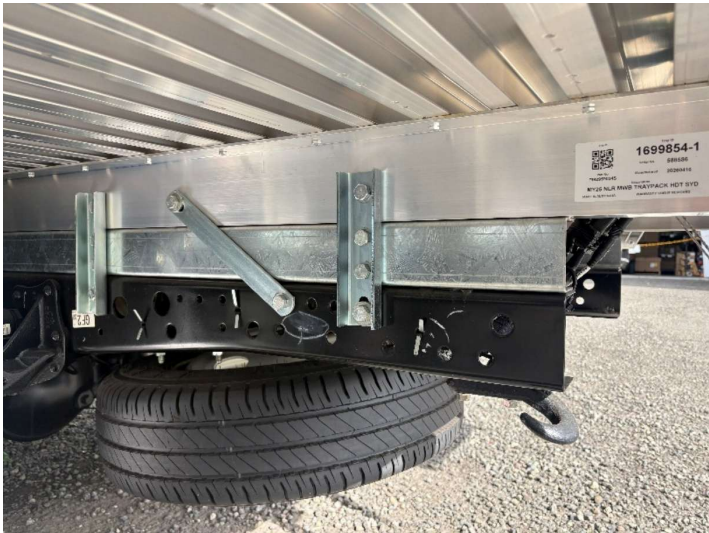
Figure 1 - Isuzu NLR TRAYPACK with reduced height chassis rails
