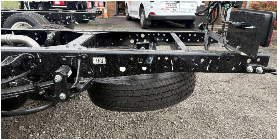
Figure 3 - Isuzu NNR Cab chassis - P/S chassis rail
